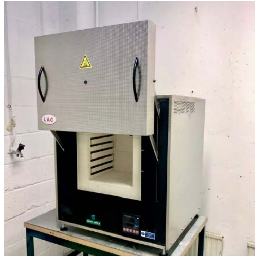
Figure 7 Furnace used in the project LAC LH15.
