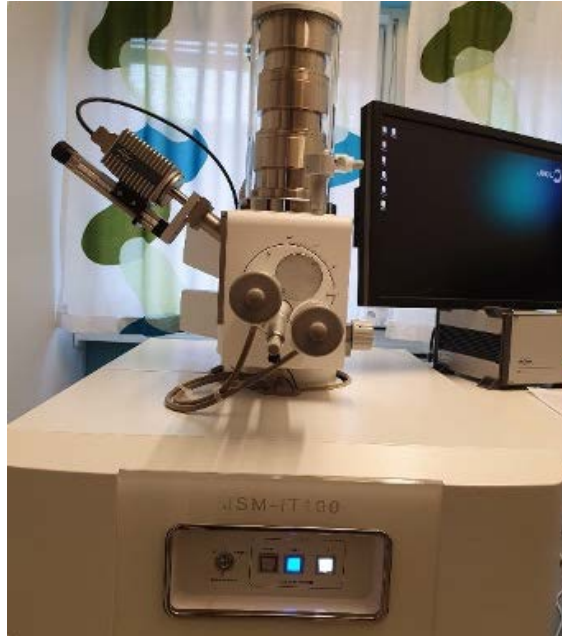
Figure 6 . SEM tyle Jeol JSMT100 used in this study.
