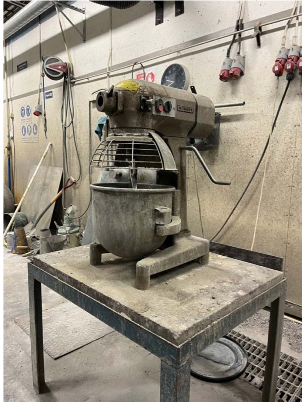
Figure 5 Mixer used in this study, type Hobart 200N
