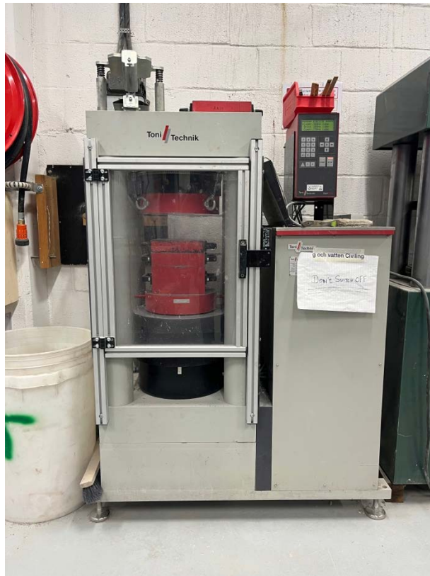
Figure 9 Compressive strength machine used in the project
